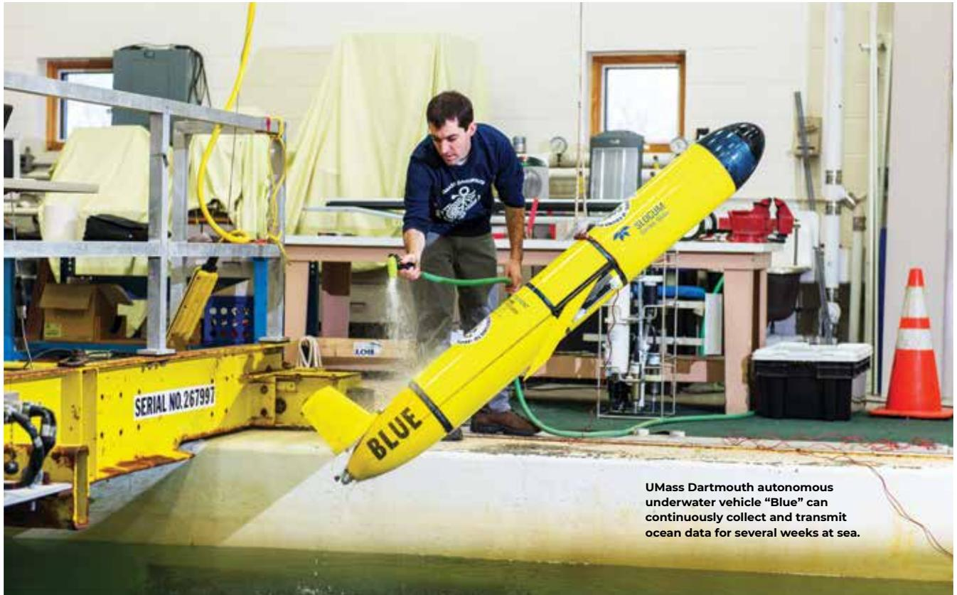
UMass Dartmouth autonomous underwater vehicle “Blue” can continuously collect and transmit ocean data for several weeks at sea.
